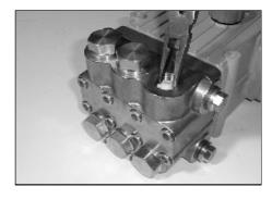
2) Using needle nose pliers, remove the inlet and discharge valve assemblies (27A). Note: It may become neccesary to remove the valve seat (27) from the valve casing using a slidehammer.
