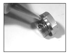
4) Remove the o-ring (31). Inspect all parts for wear and replace as necessary. Apply one drop of loctite 243 to the valve plugs (32) and tighten to 125 ft. lbs. (170 Nm).
