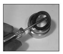
8) Remove the weep grooved seal (23) out of the seal adaptor (20). Check O-rings (21). **IMPORTANT!** The grooved seal (23) on the high-pressure side is to be fitted carefully into the valve casing (26) using a screwdriver. Under no circumstances must the seal surface in the valve casing or the seal lip be damaged.
