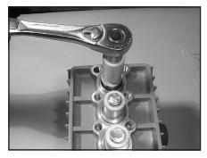
10) If the plunger pipe (16B) is worn, remove tension screw (16D) and remove along with plunger pipe (16B). Check and clean plunger surface (16A), check oil scraper (16H). Cover thread of tension screw (16D) with a thin film of Loctite and tighten carefully to 247 in.-lbs. (28 Nm).
